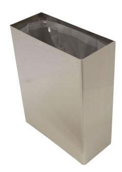
Model WA7042 is our large wall mounted waste bin, manufactured from grade 304 stainless steel polished to a satin finish. Suitable for wall mounting all edges are hemmed at top and bottom for safety. The bin is provided with four interior hooks for attaching the removable heavy duty vinyl liner. The bin has a 26.5L waste capacity.
